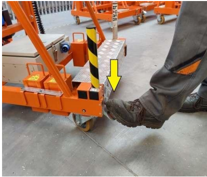
Figure 5. Wheel lock Press the pedal to lock
