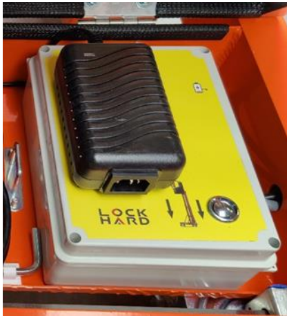
Figure 19. Electric lowering system
