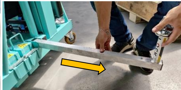
Figure 9. Pulling out the feet from the socket
