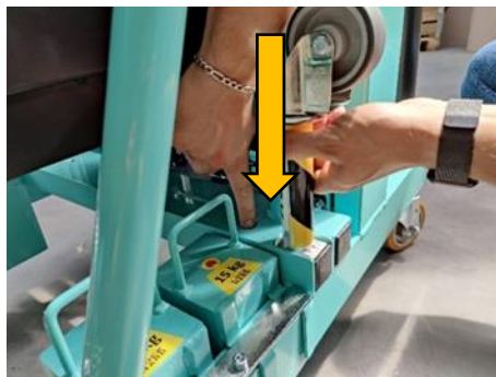
Figure 8. Pressed locking pin
