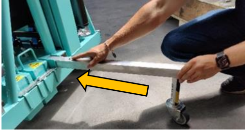
Figure 10. and figure 11. Inserting the rotated stabiliser feet
