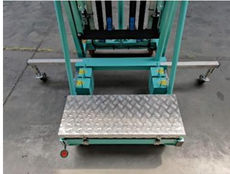
Figure 13. Unfolded the side stabiliser feet
