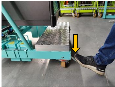
Figure 5. Wheel lock Press the pedal to lock
