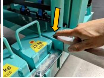
Figure 10. and figure 11. Inserting the rotated stabiliser feet
