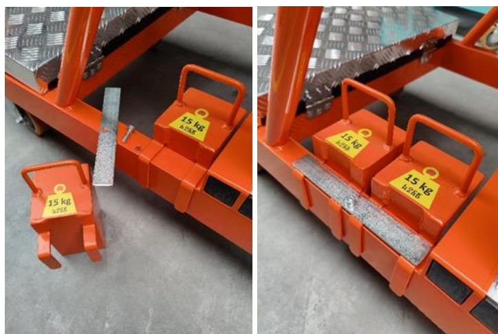
Figure 3. Installation du lestage
