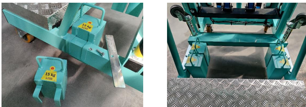
Figure 4. Installation du lestage
