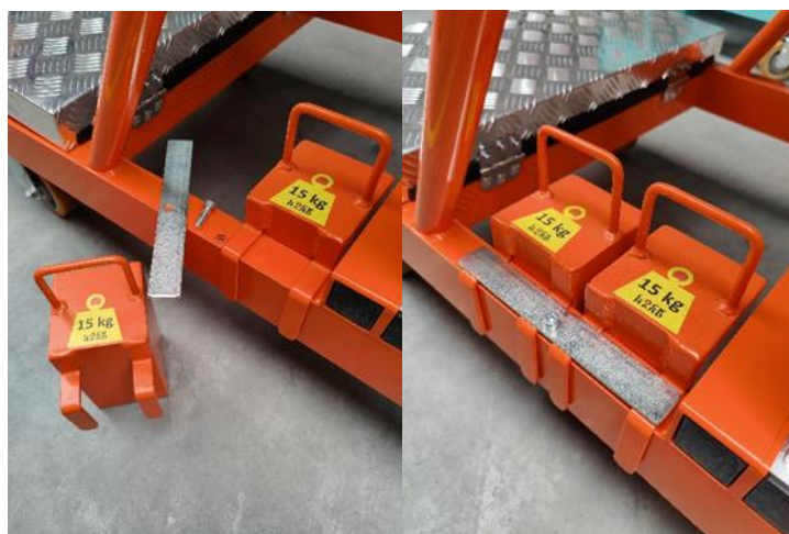
Figure 4. Installation du lestage
